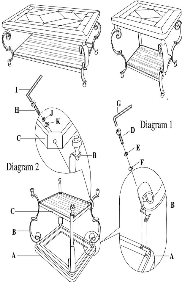
1. Place the table top (A) upside down on clean surface. Insert the washer (F) and lock washer (E) to the small bolt (D) and put the leg (B) at corner of table top as diagram 1. Make sure that the holes on leg align with the holes on top frame. Then use small wrench (G) to thread the bolts (D with F, E) through the leg bracket and onto the top. Do not tighten the bolts at this time. Repeat the same assembly for other three legs.
